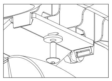
Figure 12: Securing the bottle holder in place
